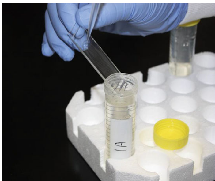
Fig. 9 Carefully position the array over a conical of wash buffer and pipet on the array to dislodge beads
